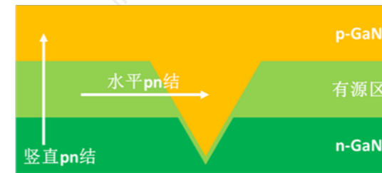
Figure 4 Schematic diagram of the 3D PN junction formed by the V-pits in the GaN-based LED
